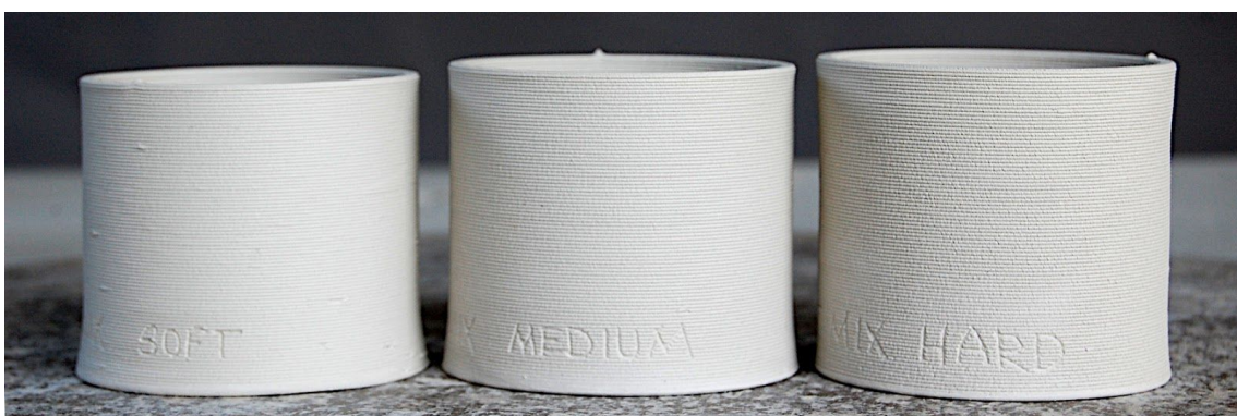
Bone dry variation in shrinkage indicating difference of water content.
