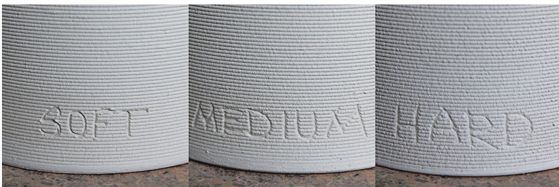
Slight variation of surface texture where the softer the extrusion the smoother the result.
