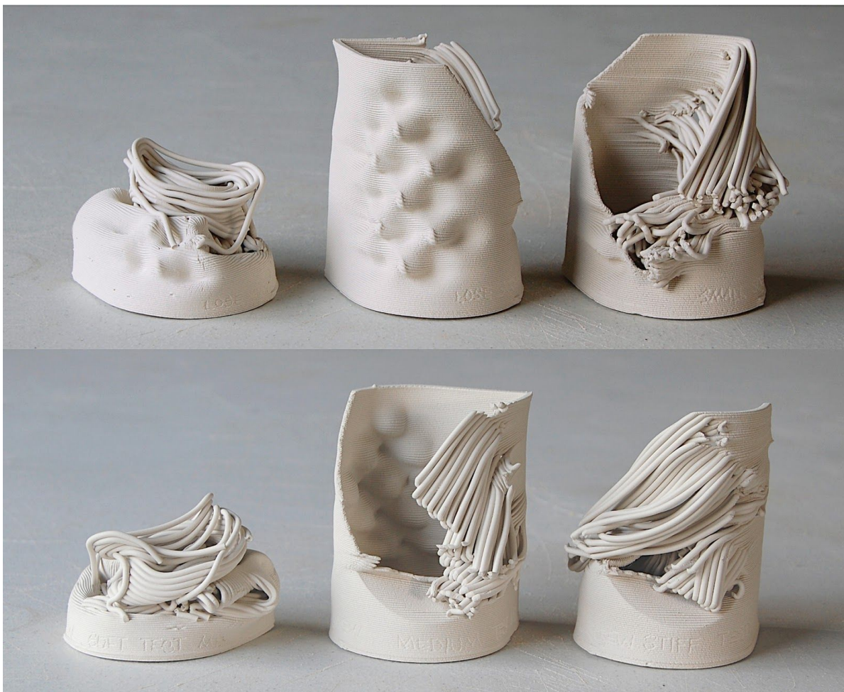
Two views of the soft, medium and hard clay print tests. Left to right - soft, medium, hard clay. Top image illustrates the repeat relief texture side of the test and bottom image the 45° angle indentations test side.
