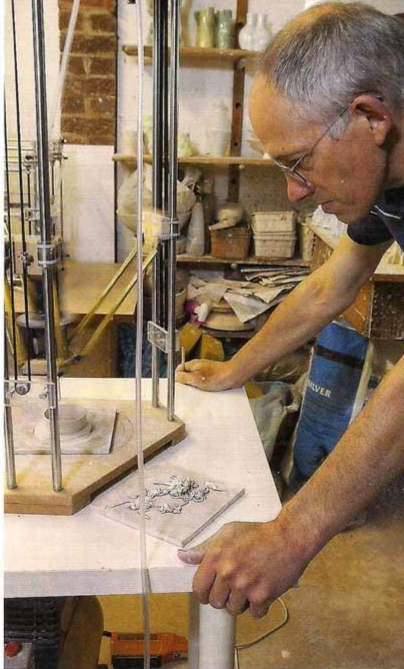
Right; Jonathan Keep using his DIY Delta 3D printer. Top; inside Jonathan's studio. Above and left; artworks created using the printer. Far left; the printer making a bowl from a computer pattern
