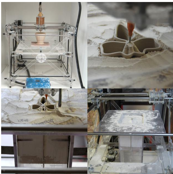
Figure 2: RepRap 3D kit printer converted for printing in ceramic. Top left: printer without powder adaption. Top right: Close up of
