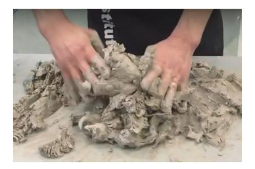
All clay can be used for 3D printing but some clays print better than others. What you are looking for is a clay that is not too sticky, that has a fine texture and dries quickly. If you are using a printer with a screw printhead do not use anything that is too rough or you will wear the screw in the printhead.
